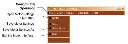
Figure 2.6.2: SPI Motor Interface File Menu
